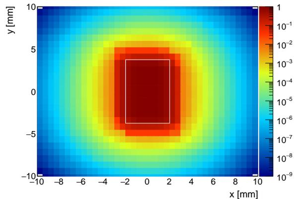
Figure 1: Pad response function of an Inner Readout Chamber of the ALICE GEM TPC for different start points of the electron avalanche. The white lines indicate the outline of the pad.
