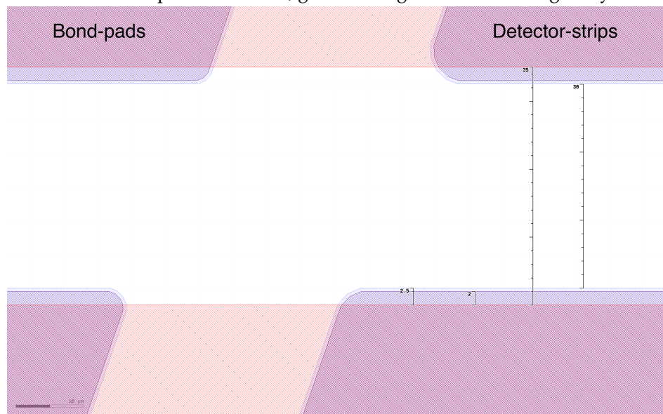
(b) Top-view on the final detector design. Reddish areas show the p-implant. Blue shaded areas represent the metallisation and purple areas the mask for the compensation oxide. Distances are given in \mu\text{m} .
