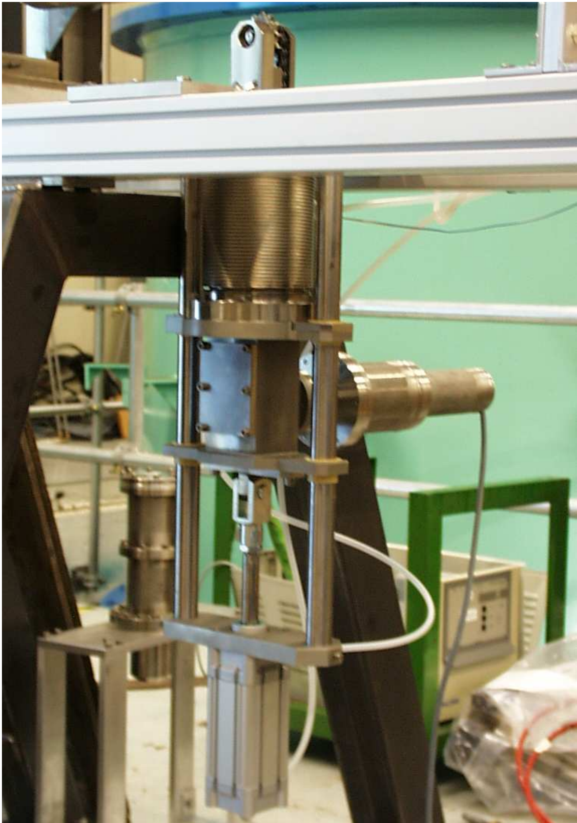
Figure 7.20: Picture of the retractable motor unit. The stepper motor is encased in the smaller stainless steel cylinder to the right. The larger cylinder contains the magnetofluid coupling. A bellows and a pneumatic cylinder are required for retracting of the motor.
