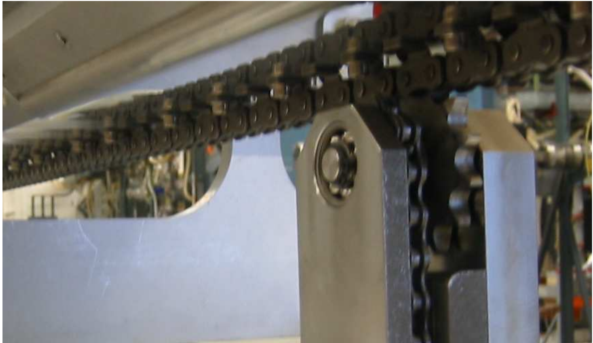
Figure 7.16: Picture of cog wheel engaging the transmission chain. Due to the pointed teeth of the cog wheel it meshes very smoothly with the chain.
