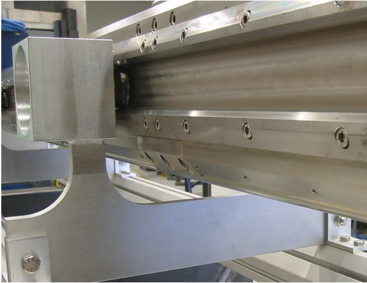
Figure 7.15: Picture of aluminum support structure, with guiding rolls, simulating the situation in the beam tube.
