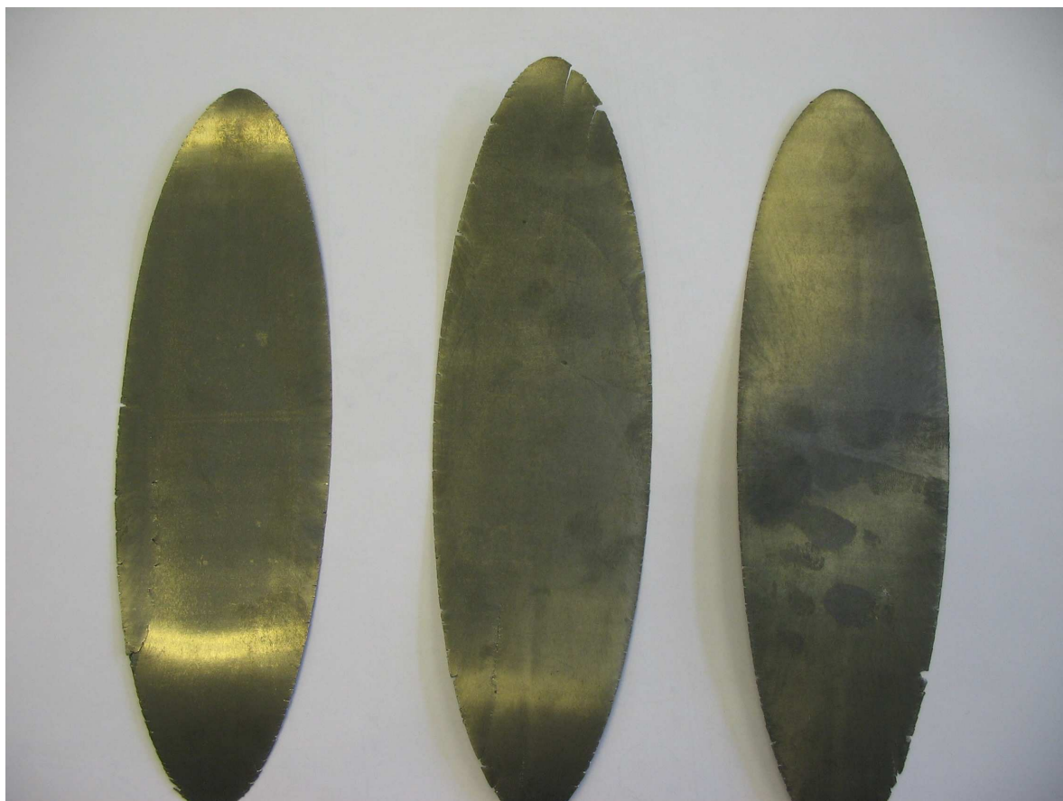
Figure 7.29: Photograph of the Gd after milling. The brittle material shows cracks occasionally.
