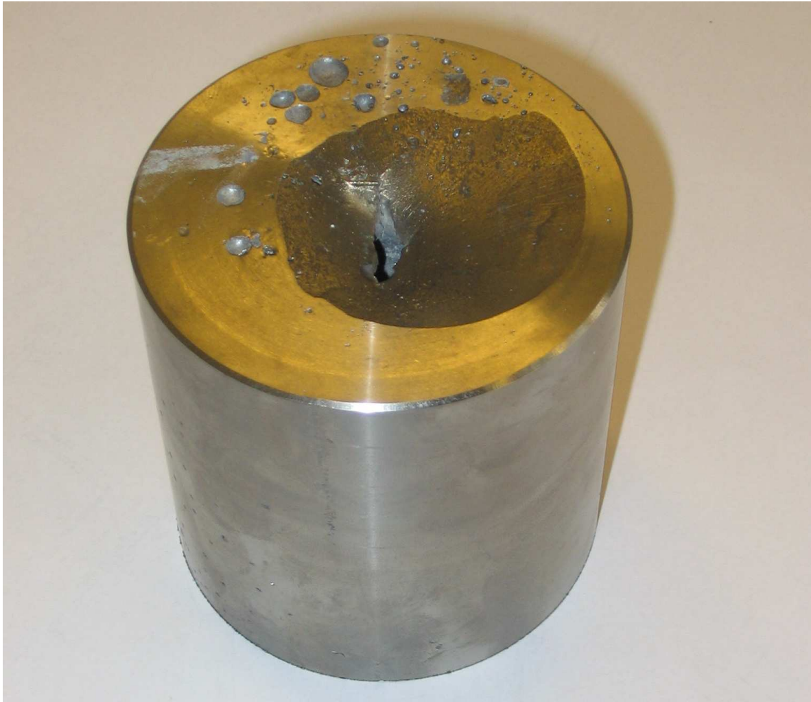
Figure 7.28: Photograph of the Gd lump after turning on a lathe. Largest crater on top preserved original coloring. Cut of sinkholes can be seen as well.
