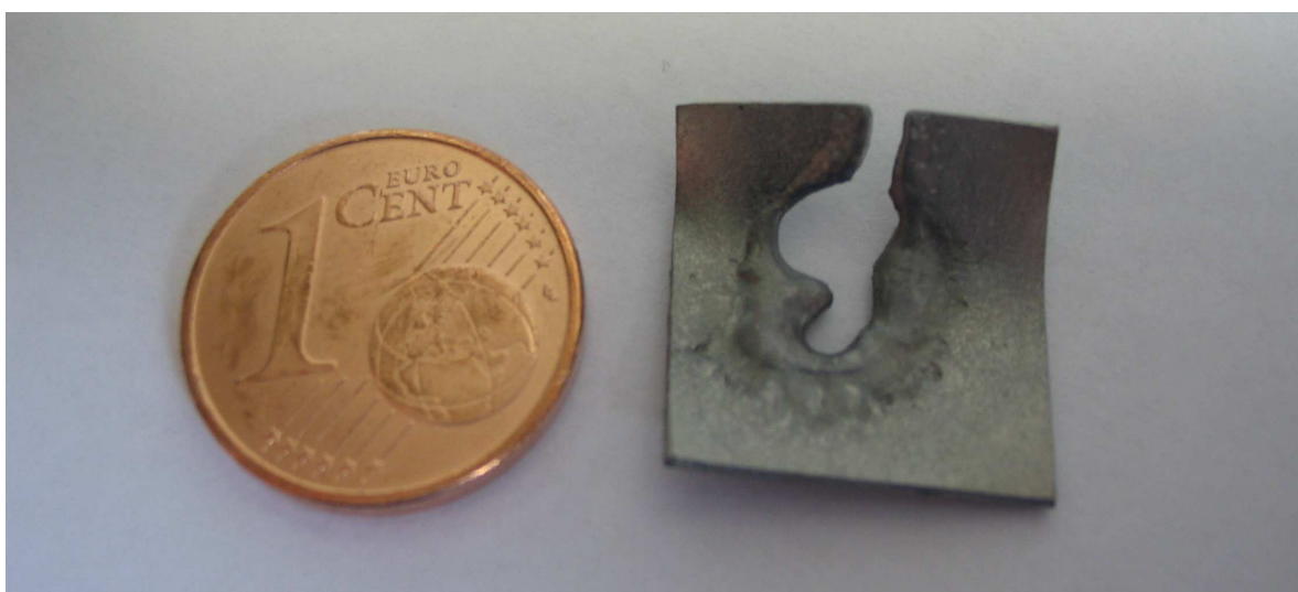
Figure 7.30: Photograph of the Gd after tempering up to the melting point. The material regained a high flexibility.
