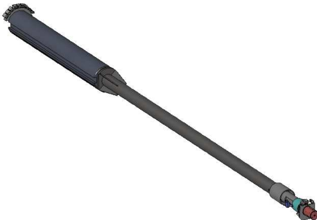
Figure 2.4: Schematic drawing of the source trolley with mounted ion source.
