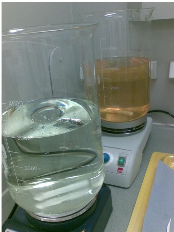
Figure 4.4.: Sample during the concentration step using  $\text{Fe}(\text{OH})_3$  co-precipitation. In the rear beaker, the pH was adjusted to 8 leading to the precipitation of  $\text{Fe}(\text{OH})_3$  whereas in the front beaker the  $\text{Fe}^{3+}$  ions are still in solution, causing the light yellow colour.
