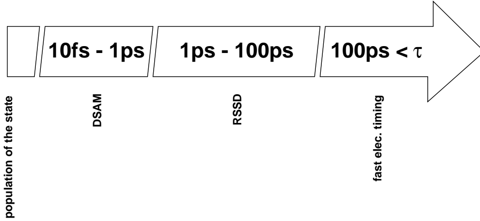
Figure 1.9: The different time ranges of methods for lifetime measurements of excited states in nuclei. The arrow indicates the time bar that is started with the population of the state of interest. RSSD stands for “Recoil Distance Doppler Shift” Method and DSAM stands for “Doppler Shift Attenuation Method”.
