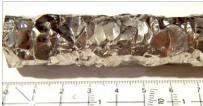
Figure 3.1.: Photograph of a metallic Zr rod. Source [21].
