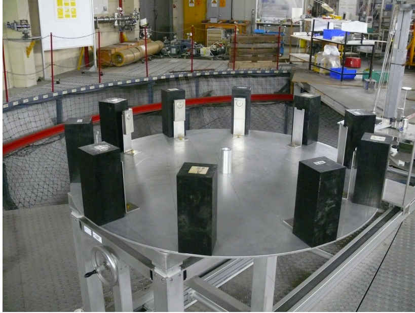
Figure 5.14.: Wheel for the simultaneous irradiation of ten dosimeters (from [25]). The AmBe source is placed on the holder in the middle; the black cubes are the polyethylene phantoms used in this setup.
