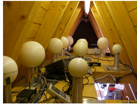
(b) Bonner Sphere Spectrometer operated at the UFS
