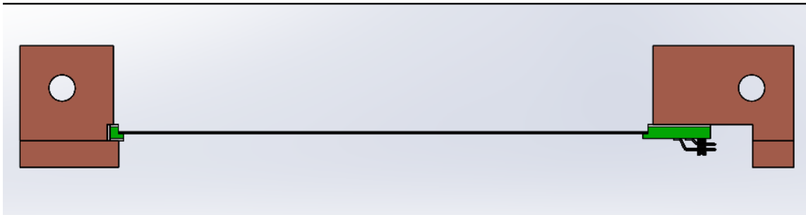
Figure 3.3: Cross-section of indirect cooling for a pion tracker detector. The cooling structure made of copper and the thermal pads (white) that are pinched between detector-PCB and cooling structure can be seen.
