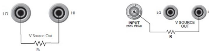
Figure 2.5: VSOC connection (left) and HRMC connection (right) [16]
