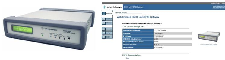
Figure 2.8: Agilent E5810A LAN/GPIB Gateway [18] and intern user interface(right)
